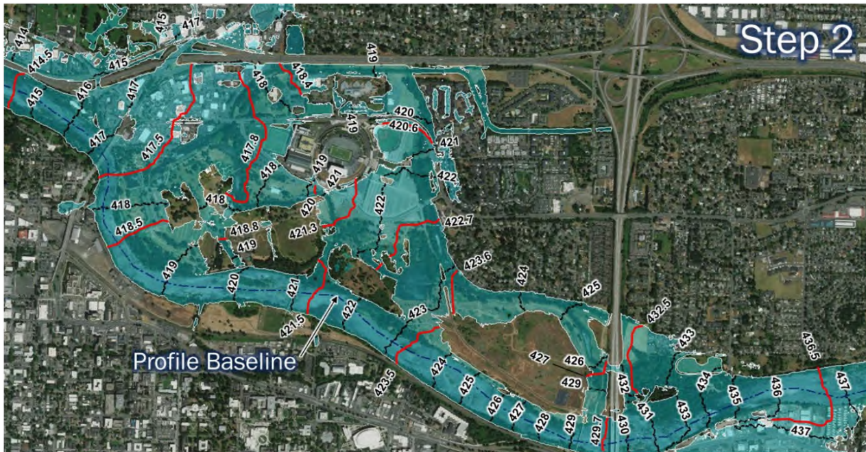
Figure 4: Sample Whole-foot and Decimal (Red) BFE Placement within a 2D Modeled Area
